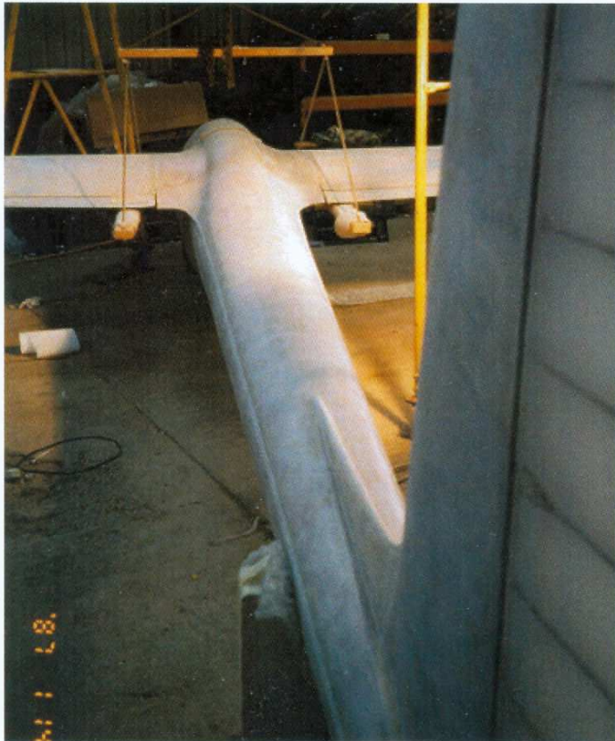
Fig. 5.8 Diatex covering on fuselage
