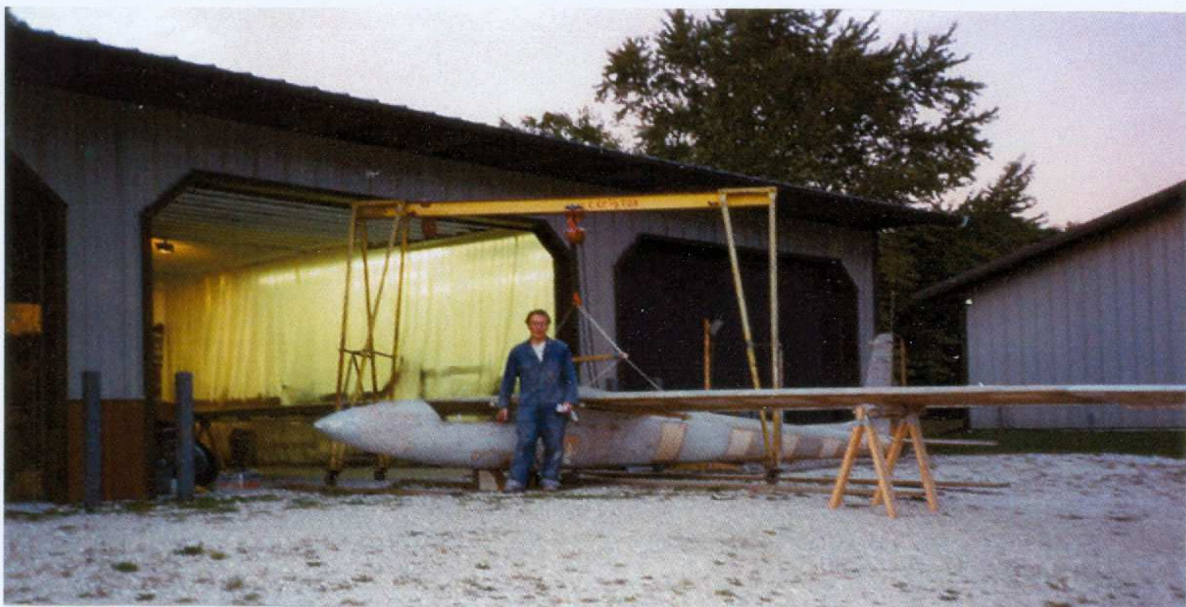
Fig. 3.11 First assembly to check controls
