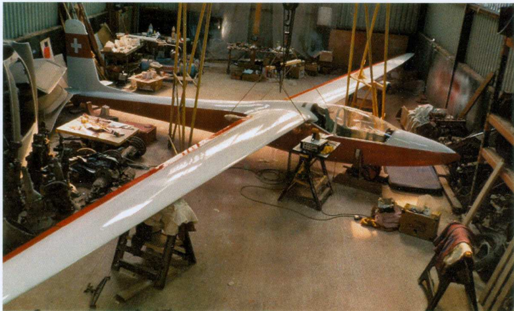
Fig. 5.13 Assembly for weighing after painting
