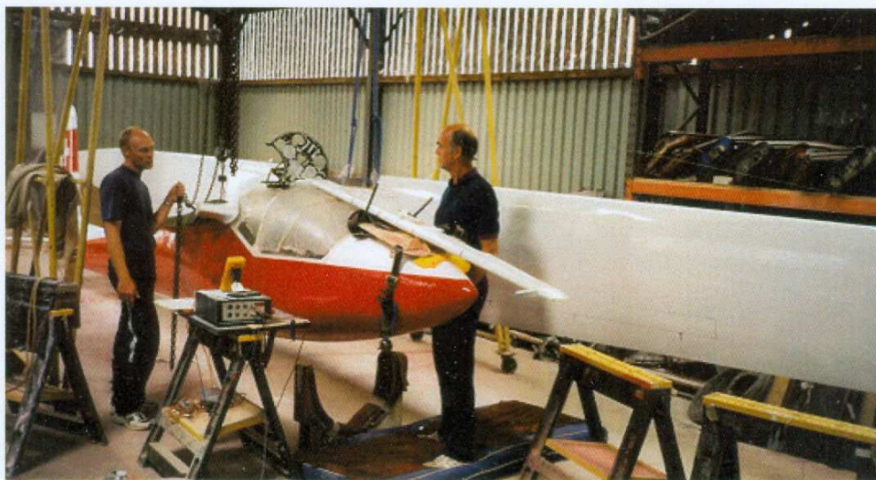
Fig. 5.12 Weighing after painting
